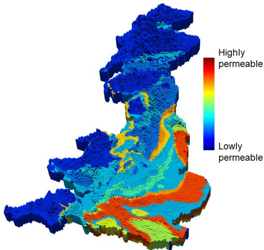
An example of input data (hydraulic conductivity) used for the current version of the groundwater flow model
