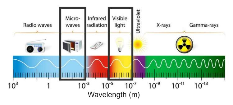
**Microwave** (MW) signal: → can go through clouds, dust, rain
